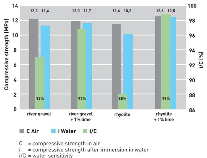
Validation using the Duriez test, NF EN 12697-12, on BBSG 0/10
